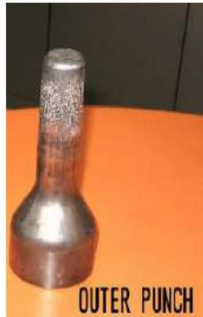
Raw material size Outer punch: 60.8mm dia
