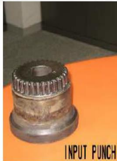
Raw material size Input gear punch: 101.5mm dia
